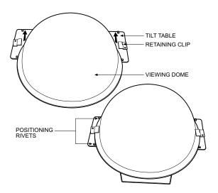
Figure 3. Acrylic Viewing Dome Installation
